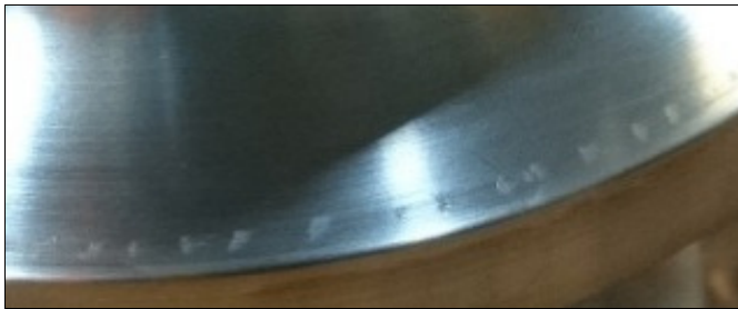
Fig. 1. Example of surface degradation of forging roller
